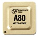
Allwinner's latest flagship UltraOcta A80 application processor is a revolutionary advance in mobile processor technology. The A80 packs octa-core big.LITTLE Cortex $^{TM}$ -A15/7 architecture in a 28nm process to deliver an outstanding combination of both computing power and efficiency.
